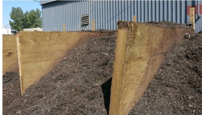
Compost curing in bunkers. Photo taken by Pam Groat
