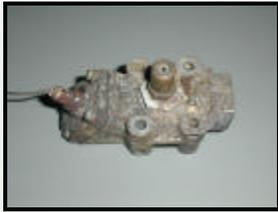
*Mercury containing pilot flame sensor removed from gas range*
