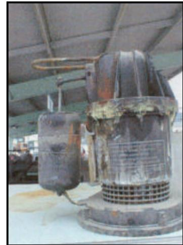
Example of a mechanical sump pump which is mercury-free. A metal guide has been used instead of a wire—this is a good indication of a non-mercury containing sump pump.
