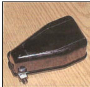
Example of a mercury containing bilge pump. Older bilge pumps use mercury to complete an electrical circuit, thus turning on the pump. Newer pumps use a steel ball. Shaking the unit can determine whether it contains a steel ball or mercury.
