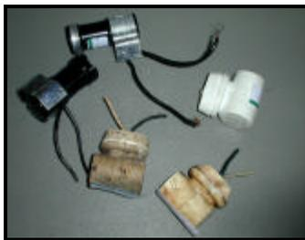
*Mercury containing switches removed from chest freezers*
